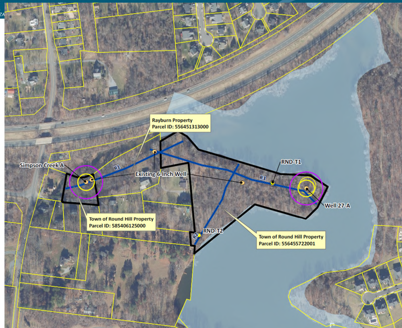
FIGURE 3 Hayman Lane Electrical Resistivity Survey Line Locations and Proposed Exploratory Test Well Locations
